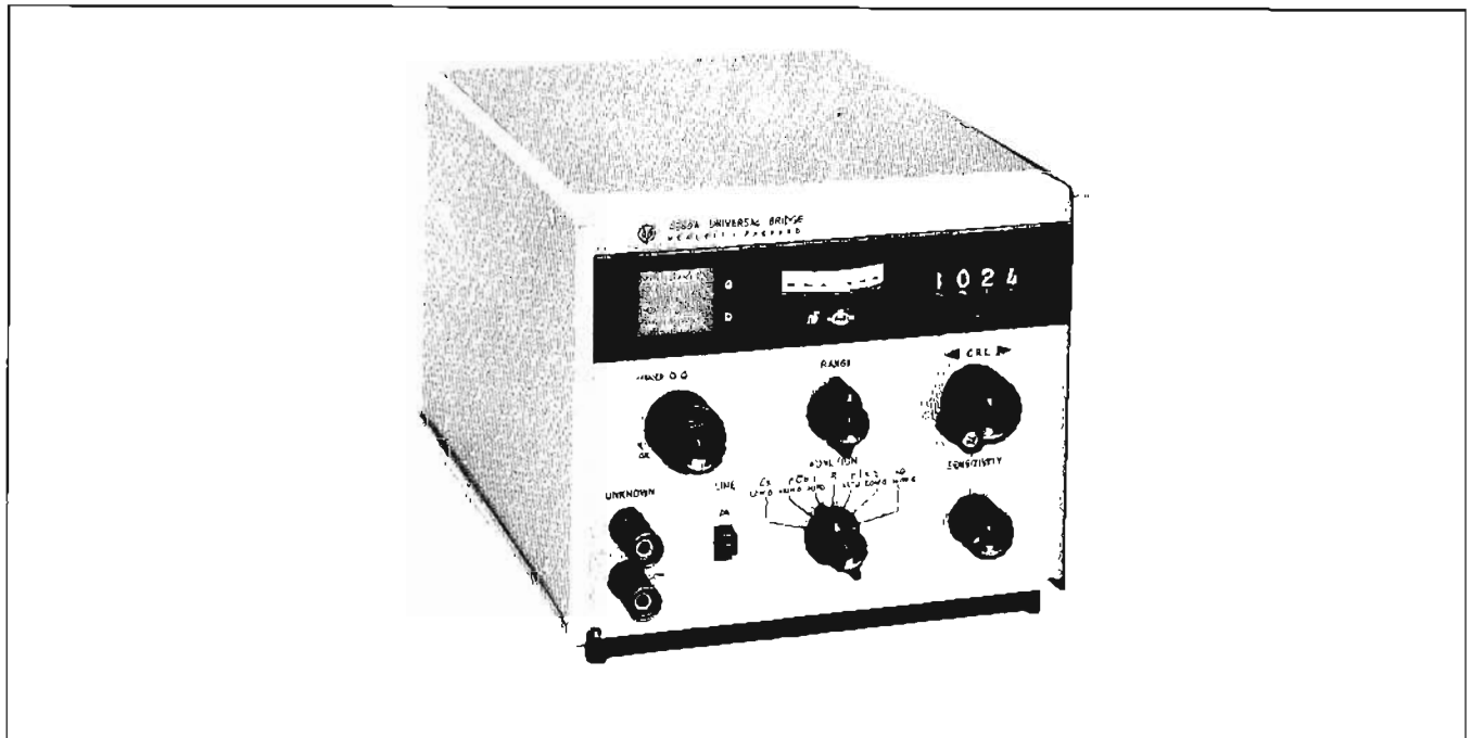
Figure 1. New Universal Bridge has digital read-out, automatic decimal placement, non-ambiguous range indication, and other features that simplify measurement of resistance, capacitance, inductance, Q, and loss factor. Bridge design eliminates prolonged balancing procedures formerly caused by sliding null in measurements of lossy relative components. Control circuitry automatically brings DQ resistor to correct value as CRL dial is adjusted for a null.
