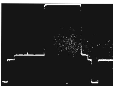
Oscillograms made with HP Model 191A TV Waveform Oscilloscope displaying Vertical Interval Test Signals; Multiburst Signal (left), Sine-squared Pulse and Bar (center), and Modulated Stairstep (right).
