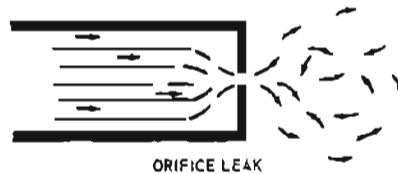
ORIFICE LEAK Figure 1
